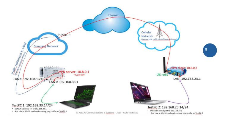
This scenario exhibits a connection from a cellular VPN client, in the field, to a VPN server at a company backbone.
